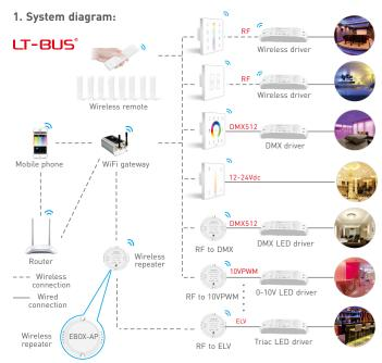
EBOX-AP wireless repeater applies LT-BUS wireless communication protocol for wireless signal
