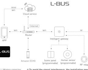
\* To avoid the signal interference, the installation needs to keep away from the large area metal material or the metal material space.
