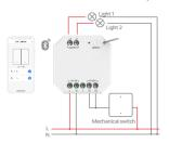
4. One push switch controls two relays.
