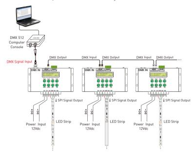
6.4 Connected with DMX 512 manual console, realizing DMX administrative function.
