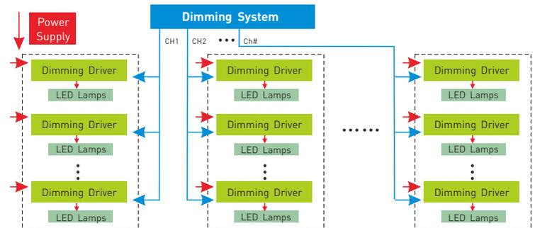
5.2 Connected to LEDs:
