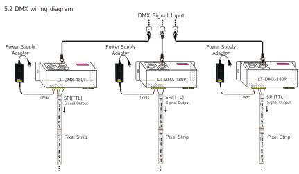
\* An amplifier is needed when more than 32 decoders are connected, signal amplification should not be more than 5 times continuously.
